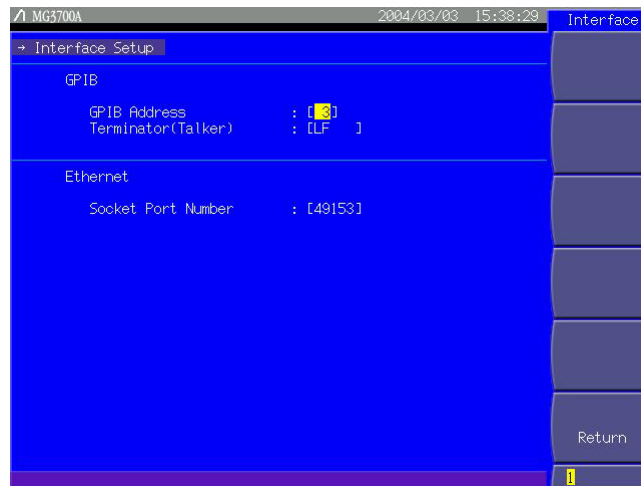
Fig. 4.2.1-2 Interface Setup screen (for GPIB interface conditions)
